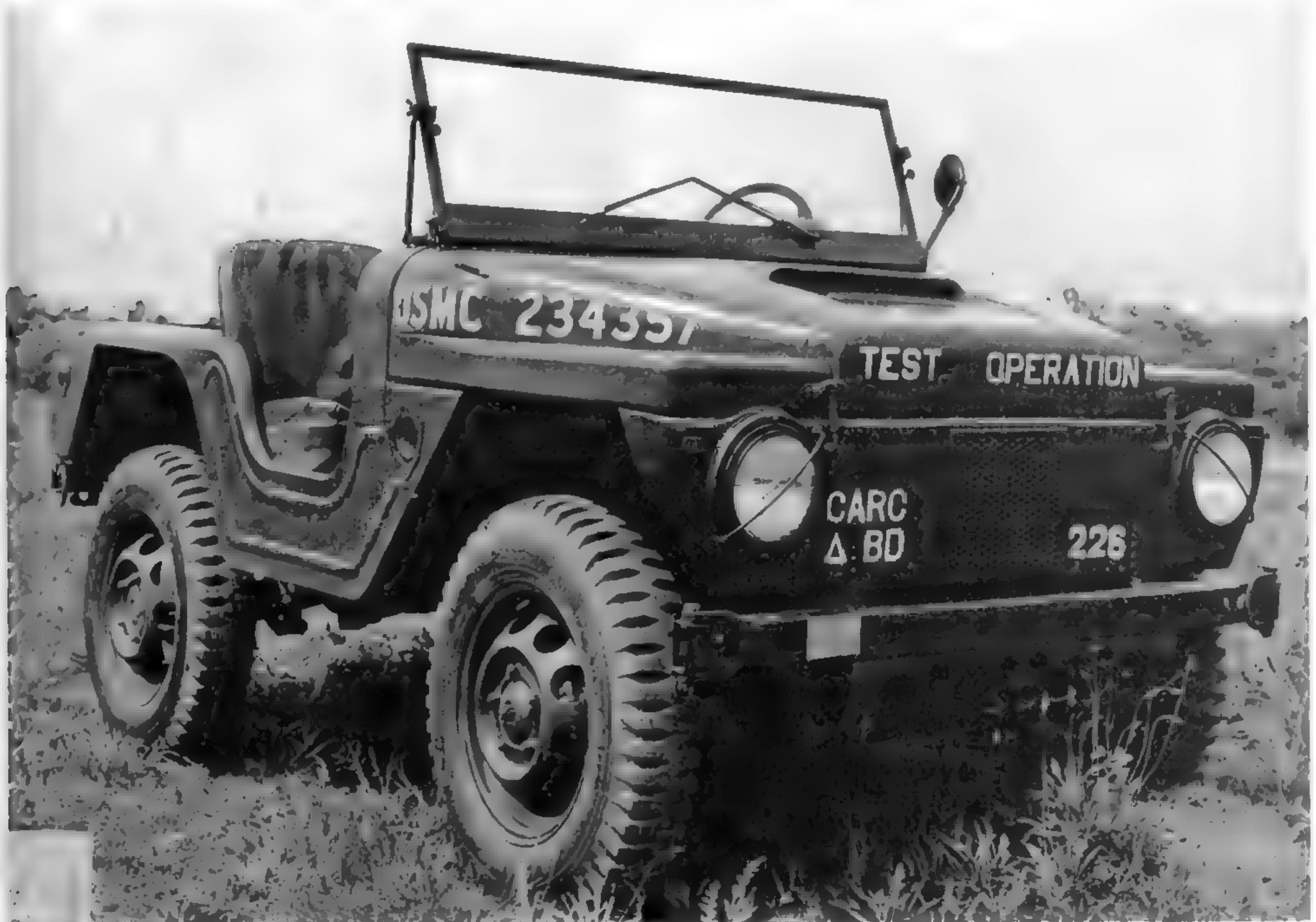
The initial production Mighty-Mite, the M422, was noted for its short length, tight turning radius, and minimal weight. It had an aluminum body and every component was designed with optimal weight savings in mind. (Photo courtesy of the Patton Museum)
